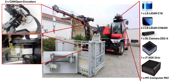
Figure 1. Robotic telehandler retrofitted into a ROS2-enabled robot with multimodal sensing. Other sensors shown besides the additionally added encoders are not exercised in this control study.
